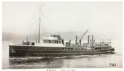
fitted with 3-96 B.H.P. Gardner Heavy Oil Engines of the direct reversible type. (For further details see over).
